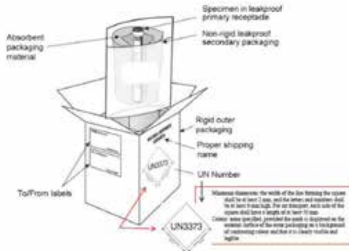
Gambar 4.10 Contoh Pengemasan Tiga Lapis Sumber: WHO-Guidance on regulations for the transport of infectious substances 2019-2020
